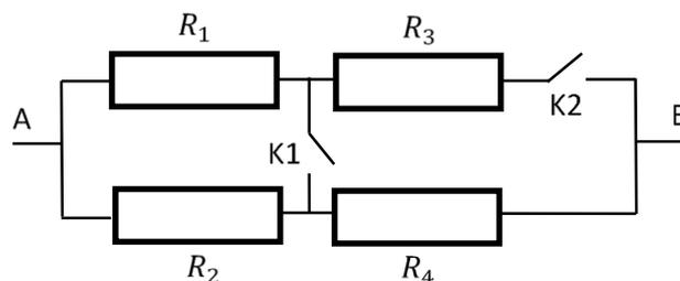
From the available experimental data, calculate the values of the resistances of the four resistors in the circuit and the initial state of each of the two switches. Fill your answer in the table below.
